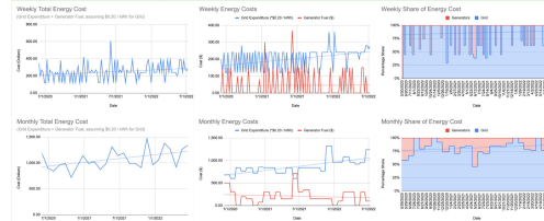
Figure 4 - mashup of hospital grid & generator expenditure data depicting total energy expenditure, individual energy expenditures, and the share between the two over the time period from 05/30/2020 to 07/09/2022.
